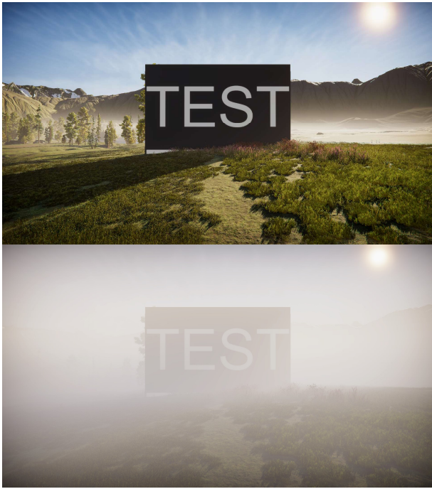
Figure 2. Test image used to measure visibility in foggy environments. The visibility distance in fog (bottom) is computed as the distance at which the contrast between the white text and black background of the test image drops below 5% of that measured with no fog (top)
