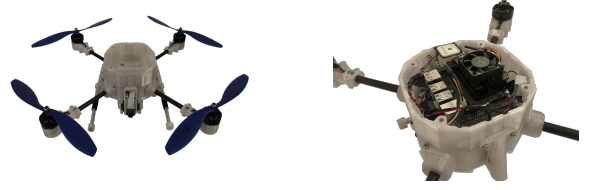
Fig. 4: Our 3D printed modular unmanned aerial vehicle (UAV). In the left picture, the complete quadrotor without the batteries is demonstrated, while in the right one, the Nvidia Jetson nano and the global navigation satellite system (GNSS) module are shown.
