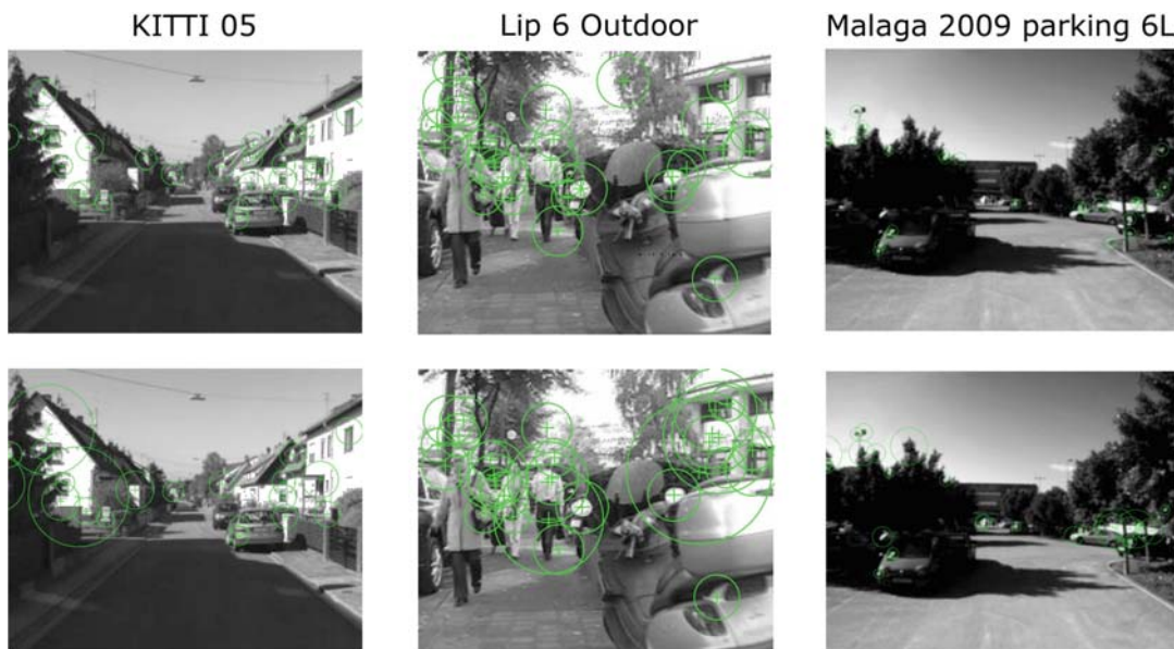
Fig. 6. Different local features extracted for the proposed method (top) and its baseline version (bottom) on KITTI 05 [18] (left), Lip 6 Outdoor [1] (center) and Malaga 2009 Parking 6L [8] (right) datasets.
